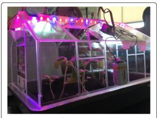
**Fig. 1** A typical example of a completed smart greenhouse. The lights, microcontroller, and battery are placed on the exterior, whereas plants, sensors, and most actuators (fans, pumps, etc.) reside in the interior
